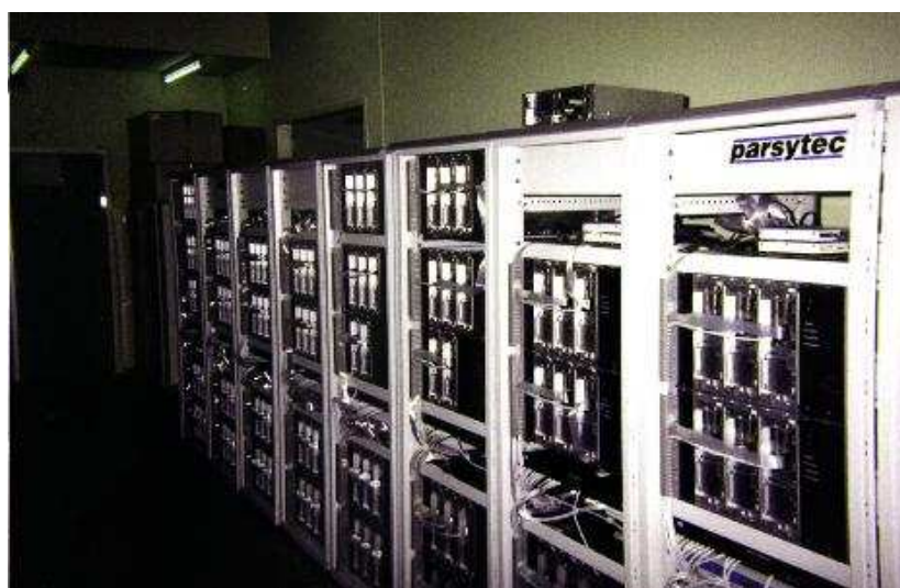
Figure 3: The Betacluster: 128 Pentium Pro PCs connected by Myrinet.
