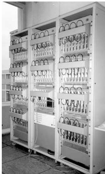
Figure 2: The Zoo: 80 single-board computers (MicroSparcs) connected by Ethernet.
